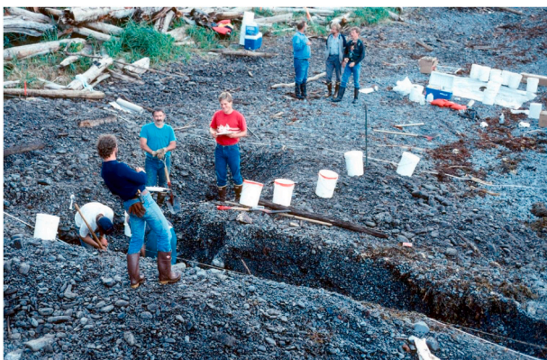
Fig. 2. Sediment hydrocarbons sampling trench 18 months post-‘Exxon Valdez’, North Latouche Island, Prince William Sound, September 4, 1990 (E. Gundlach).
