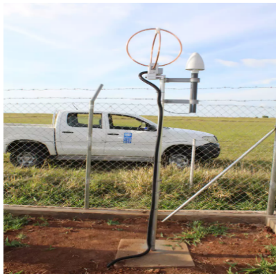
Deployment of a lightning detection sensor
