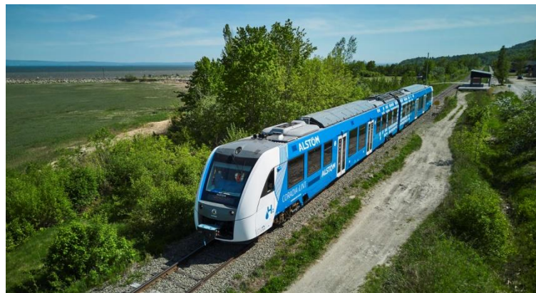
Figure 3. Successful trial operation of the world's first two hydrogen trains was officially completed at the end of February. Two pre-series trains of Alstom's Coradia iLint model have been in passenger service since September 2018. [ https://www.alstom.com/press-releases-news/2023/10/alstom-concludes-successful-demonstration-first-commercial-service-hydrogen-powered-train-north-america ].
