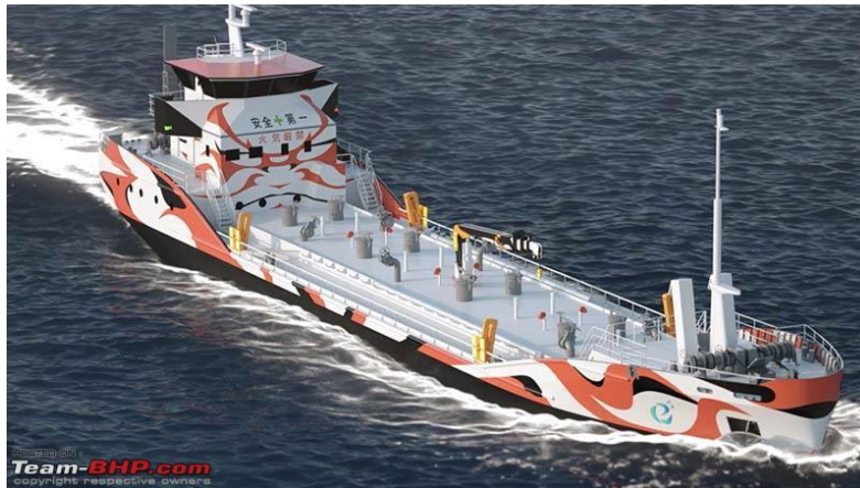
Figure 4. A Japanese consortium is designing a prototype of an all electric oil carrier ship powered by a 3500 Kwh battery. This ship, smaller than a typical cargo liner, would be 62-metres in length and have a payload of 1300 cubic metres of oil. This would serve as a proof of concept prototype before Japan embarks on full sized oil tankers. [ https://www.team-bhp.com/forum/commercial-vehicles/228455-cargo-ships-powered-renewable-energy-sources.html ].
