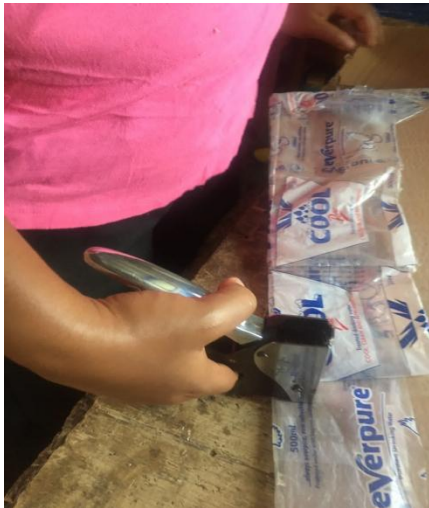
Figure 6. Clipping of water sachets with the stapler
