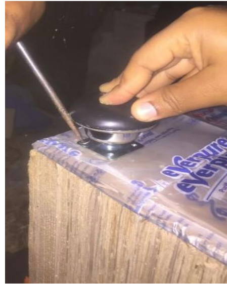
Figure 18. Fixing of stand for couch Source: Studio Work, 2021.
