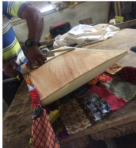
Figure 11. Clipping fabric around foam and plywood with stapler
