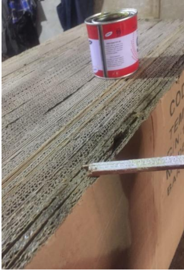
Figure 14. Stacking of boxes for couch with glue Source: Studio Work, 2021.
